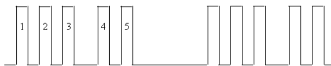
Fig. 24 Characteristics of Acoustic Alarm Signal for Patient Alarms
