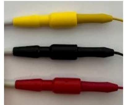
Fig. 20 Colour-Coded Sockets on the ECG Patient Cable's Distributor
