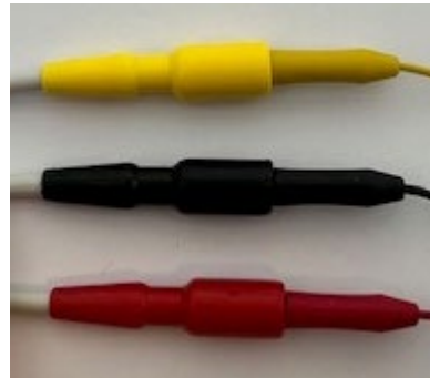
Fig. 33 Colour-Coded Sockets on the ECG Patient Cable's Distributor
