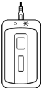
Figure 12 - Charger Pad - not charging
