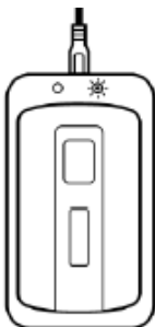
Figure 11 - Charger Pad - not charging
