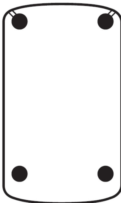
Fig. 4 Back of the recorder with electrodes
